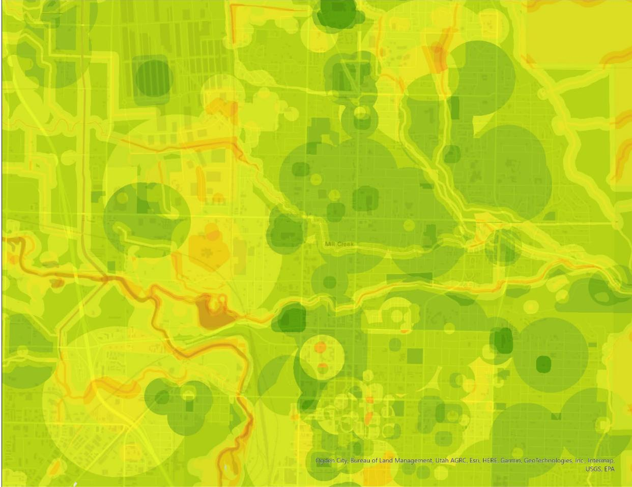
**Figure 4-8: The suitability analysis for Ogden.** Areas in red have a poor suitability, and green have high suitability. In Ogden the primary reason for reduced suitability is connection to waterways.
